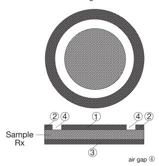
Depending on the connection wiring the RESISTOMAT® 2408 makes it possible to determinate the surface or volume resistance of the test sample.
